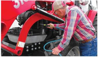
Wand tubing on the Radiator Genie is small enough so you can get into confined areas, yet big enough to create a lot of force with air or water.
