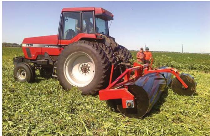
Roller’s chevron pattern grips the ground to reduce bouncing. Each roller has 23 angle irons mounted at 8-in. intervals, with the edges welded to the roller.
