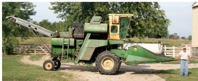
David Newbury converted a 1960’s Deere 55 combine into an ear corn picker equipped with a 3-row header. Elevator unloads out the back.
