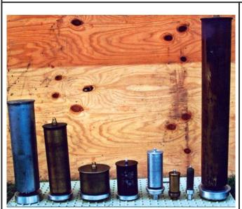
Dave Dam turns old artillery shells of various sizes into steam whistles. Air goes up through the bottom, and a plate forces the air to move up the sides which causes the shell's upper chamber to vibrate.
