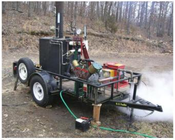
Trailer-mounted, steam powered generator runs on wood or anything else that burns.
