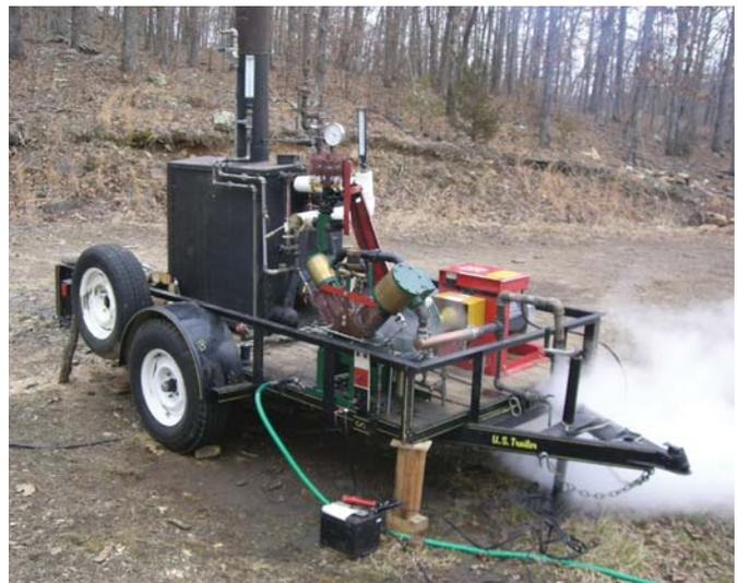
Trailer-mounted, steam powered generator runs on wood or anything else that burns.
