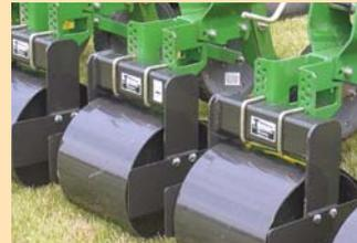
Crop slides between rollers, which are equipped with metal shields on both sides.
