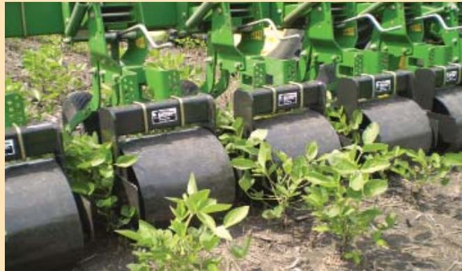
Each roller is 16 in. dia. and has a clamp-on toolbar mounting bracket on front.
