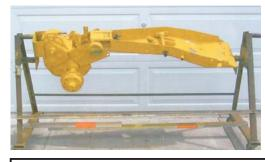
He uses this stand to work on garden tractors. It has adjustable mounting brackets at either end.
