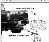
with bead breaker, mount/dismount bars, etc. I take it with me on road trips where I almost always blow a tire or two. I welded a 2-in. sq. tube on the tire changer assembly that fits into my pickup's receiver hitch. I also welded an extra receiver tube on the tongue of my trailer, which allows me to change tires on the road without having to drop the trailer. It works great and has saved me a lot of money over the years."
