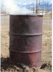
Barrel stands in a shallow hole. Note small opening, lower right, to let air into bottom of barrel.
