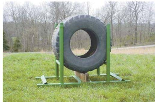
**Big floatation tire sets in a cradle built out of oilfield pipe. It rides on runners made from 4 and 6-in. well casing.**
