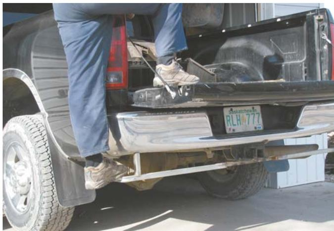
**"Easy step" bumper attachment bolts to pickup's receiver hitch and also to bumper.**
