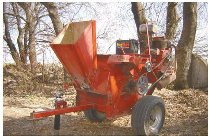
**Portable wood chipper is built out of an old Gehl silage chopper. A Kohler 14 hp engine belt-drives the chopper's rotor.**
