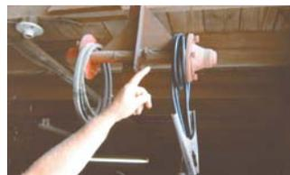
"I used a pair of wheel hubs to hang up the terminal clamps on my electric welder. First I welded an old tractor spindle to a length of angle iron, and then I welded both hubs to the ends of the spindle. Then I lag screwed the angle iron to the wall in my shop. What's nice is that all edges are rounded so there's nothing to catch or scratch. Also, I can unwind however much cord I want without having to drag it around."
