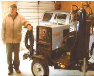
retired and moved to the country. He wanted to make certain he could take his standby power wherever he wanted, so he bought a Harbor Freight trailer and mounted a gas welder and a generator on it. The generator is set up for either 110 or 220 volts and has an output of 10,000 watts. With 110 volts it has an output of 80 amps; 40 amps with 220 volts.
