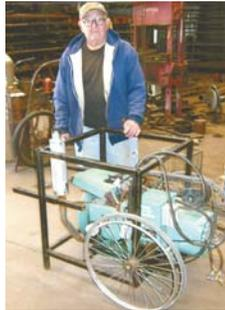
wheelbarrow. It mounts on a frame made from 1 1/4-in. steel tubing and rides on a pair of wheelchair wheels. A car exhaust and muffler help keep the noise down.
