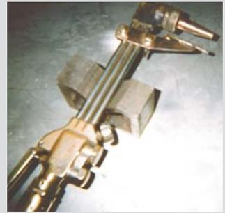
**Attachment's pointed metal rod sticks out beyond torch's cutting head. It slides up and down torch, cutting neat holes up to 12 in. in dia.**
