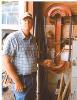
**Tom De Clerck, Pana, Ill.:** "I can store up to 200 ft. of air hose neatly out of the way with this homemade 'split wheel' holder. I cut a car wheel rim in half and welded a 4-ft. length of 4-in. channel iron to the back side of both rims. Then I bolted the channel iron to the wall. I just wind up the air hose in big loops on the rims. I mounted the unit near the door of my garage, where the air hose is readily available for any inside or outside job."
