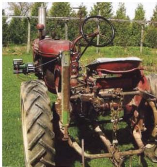
Cable runs from winch back to a clevis mounted on top of a vertical metal bar that's part of tractor's lift system.
