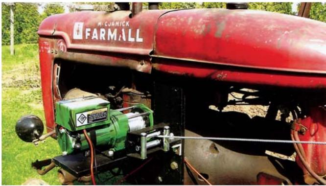
Electric winch mounts on side of tractor, making raising or lowering tractor's lift system as simple as pressing a button on a remote control.
