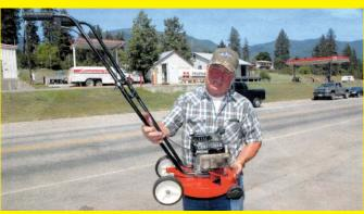
This is a 12-in. lawn mower I made from scratch because I couldn't find a small mower for use around my garden and fence. The engine came from a small rotor tiller that I found in the trash.
