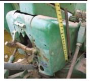
while looking back over my right shoulder. The lift lever was previously mounted on the dash and would often get stuck. I moved the lever to the back of the tractor.
