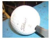
up. One day I made a file handle out of one and found it's about the best file handle you could ever have. The golf ball won't come off, and I don't get any blisters in the palm of my hand like I do with conventional file handles. I just drilled a hole and filled it with JB Weld."
