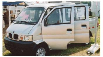
Made in China, the 4-WD, 4-door mini pickup is powered by a 4-cyl., water-cooled gas engine that gets 35 to  $40~\rm mpg$ .
