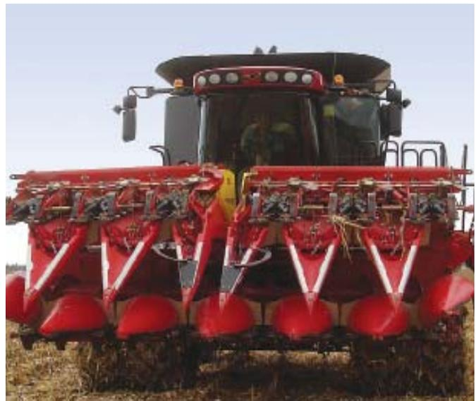
The new Capello corn head can be fitted to most combine brands and is available in a full range of models, either rigid or folding. Chopping rotors are available on all models except the 18-row.
