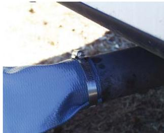
Rigid plastic adapter clamps onto vehicle's exhaust pipe.
