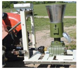
Pto-powered pelletizer has a heavierduty gearbox that'll stand up to increased pellet-making torque, says the company.
