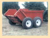
The NTH MX-8 "high lift" dump trailer rides on tandem walking beam axles and has a capacity of 8 tons (above). The box raises straight up and dumps out the back like a dump truck, allowing you to make piles up to 4 1/2 ft. high with no hand unloading (above right). With the tailgate lowered to the ground, the rig can be used to haul a skid loader down the road to the next ich
