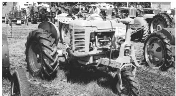
Iky Wipf used components from 4 different tractors to build this "slow speed" tractor. The 4-cyl. industrial engine — bolted crosswise on a Deere frame — is off an International Cub.
