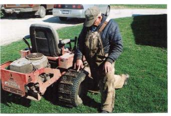
To improve traction on his zero turn riding mower, Roger Foster attached home-built channel iron tracks to the drive tires.
