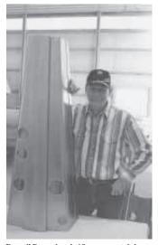
Darrell Boren bends 18-gauge metal sheets into Deere tractor hoods. He designed his own tooling to make the proper bends.
