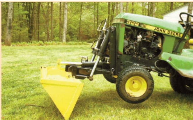
George Liskey converted a Deere model 43 front blade into this "bucket loader". Bucket's bottom and sides were made by welding 3/8-in. thick steel plate onto blade.
