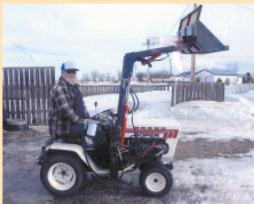
Russell Wright converted an old Roper garden tractor into a dandy loader tractor. A belt-driven hydraulic pump on one side of tractor is used to raise and lower the bucket and also to tilt it.
