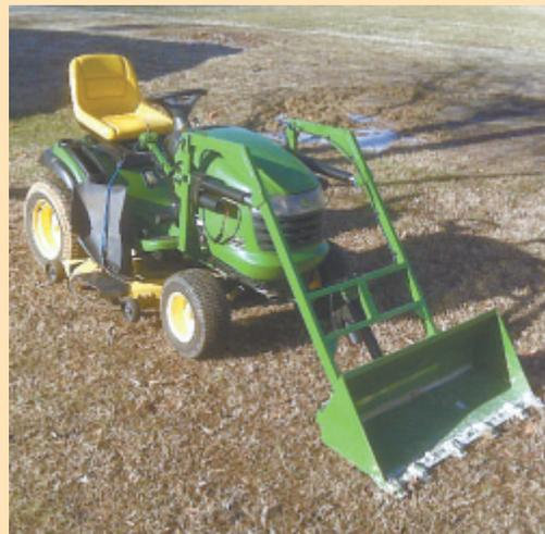
receiver hitch. It has a lift capacity of 500 lbs. and is operated by a self-centering toggle switch that mounts on the tractor's dash.
