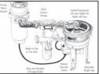
Under-the-sink food waste recycler gathers ground-up food from disposal and uses centrifugal force to separate out the water. Water goes down drain, and the food is held by the removeable basket inside unit.
