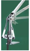
The Jack Jaw T-Post Extractor works like a ratchet on a jack. except that it grabs the post using a pair of camshaped, hardened steel jaws.
