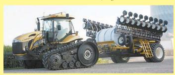
Active hydraulic down pressure provides uniform depth control in varying field condi-
