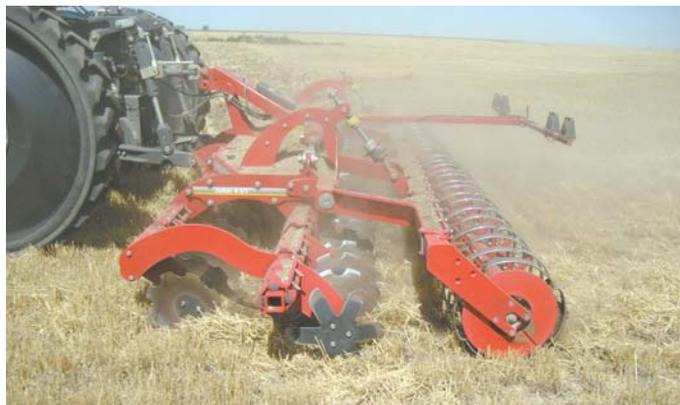
Joker compact disc combines speed with shallow tillage. It has 18-in. dia. notched blades on front and a RollFlex system at rear that smoothes the surface.
