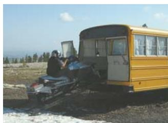
Homemade ramps hook onto bus's rear bumper, allowing machines to be loaded through double doors at back. Driver's seat was replaced with a swivel bucket seat and behind it is a reversible, double passenger airplane seat.
