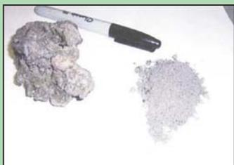
Typical clinker formed while burning hay pellets (left). Stove's ash remover reduces such clinkers into a fine powder ash (right).
