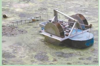
Remote-controlled, electric-operated Styrofoam pontoon is equipped with a 2 1/2-ft. wide aluminum "robot" rake. It moves about 10 ft. every 30 seconds.
