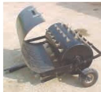
Unit's sharp sickle knives are protected by a metal cover.
