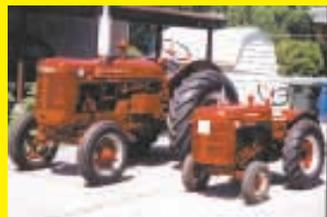
long by 3 ft. high and is powered by an 8 hp Wisconsin rope start engine. A 12-volt generator mounts alongside the engine.
