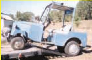
angle gearbox reverses the rotation of the engine, which pto-drives a 3-speed standard transmission off a Chevy pickup. A pto shaft off a Bush Hog mower hooks up to the cart's rear end. The rig has a tilt steering wheel out of an Oldsmobile car, as well as a chrome grill, headlights, and tail lights. Its seat is a piece of plywood covered by foam rubber padding. Top speed is 25 mph.
