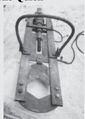
Jim Pardoe automated a long-handled dehorner by mounting the guillotine blades in a frame that's powered by a 1/2-in. drill.
