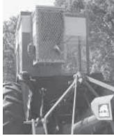
Swamp cooler mounts on back of tractor cab and is powered by tractor's 12-volt battery.
