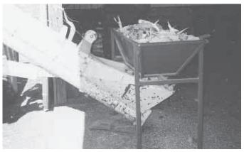
Hopper is about the width of a loader bucket and has an opening at the bottom. It keeps elevator full without overloading it.
