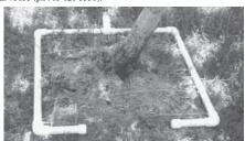
Weep holes in U-shaped pvc pipe allow water to seep slowly into
