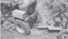
Battery-powered electric winch provides lift on the 3-pt. hitch chassis.
