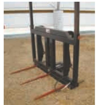
Bale fork has three tines attached to a moveable steel bar that can be extended or retracted up to 8 in. by a hydraulic cylinder that mounts on a separate bar.
