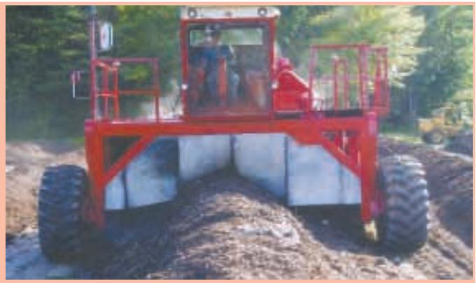
Turbo-powered 175 hp engine is big enough to turn composter's 14-ft. long beater through a windrow 12 to 14 ft. wide and 7 ft. high.
