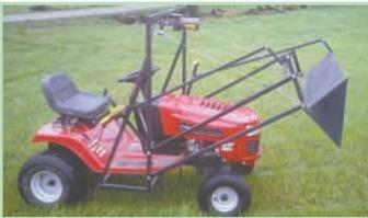
Larry Walton built this front-end loader for his Murray 15 hp riding mower. It can be raised up to 50 in, high and dumped.
