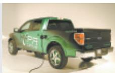
Electric F-150 is recharged by wheel motors, and by plugging it in through the fuel cap.
