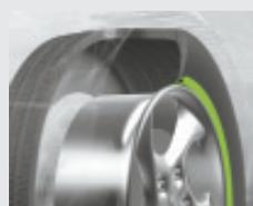
Air tube between tire bead and rim (shown in green) pumps air into tire to keep it full.
