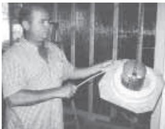
**John Marley, Athens, Ill.:** This homemade dispenser for electric cable really saves time and effort. It consists of a piece of plywood with a bottomless gallon can bolted to the center of it. The plywood and can hang from the ceiling by a chain that attaches to the center of the board. A roll of electric cable
