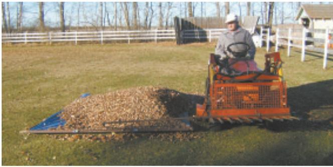
Mel Primrose drags an 8 by 10-ft. nylon tarp along one side of his riding mower to catch leaves as they're chopped up by the mower deck.
