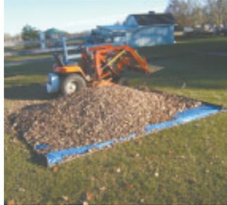
Metal bar extends out from tractor loader to hold tarp.
