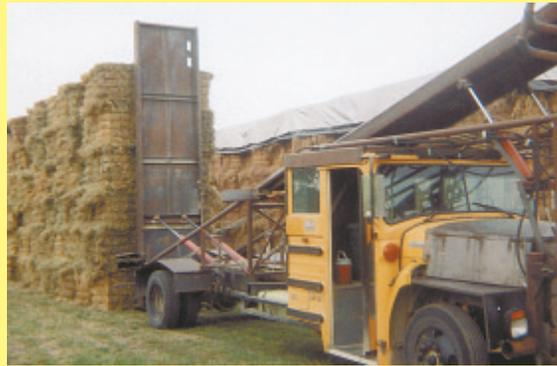
Unit can stack 3 by 3-ft. bales six high, and 4 by 4-ft. bales four high. It can also be used to retrieve the stacked bales.
