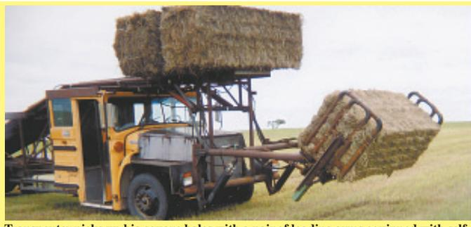
Transporter picks up big square bales with a pair of loading arms equipped with self-centering clamps.
