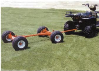
Running gear comes with a 4 by 8-ft. steel frame bed with stake pockets. The customer adds his own bolt-on plywood deck and sideboards.
