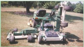
Pull-type mower is equipped with a "fake" middle deck that looks like a third mower tually the power source for two wing decks.
