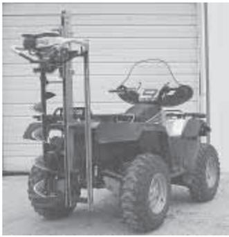
"Auger mount" transports augers and holds it while you dig. It can be used on both ATV's (left) and pickups.
