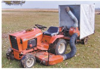
Snowblower's vacuum fan and cage mount on the frame of a 2-wheeled enclosed trailer.
