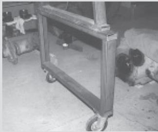
ing height of his A-frame hoist. His solution was to build two rectangular frames and weld them onto each side of the A-frame, adding a pair of caster wheels on each side. The frames added an extra 3 ft. of height."
