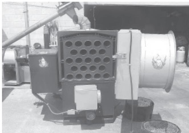
Randy Severson's 600 Rocket furnace introduces combustion air from the top, which allows the furnace to burn corn at a very high temperature.
