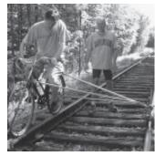
Skate wheels in a bracket attached to front wheel run against each side of rail, holding the bike in place.
