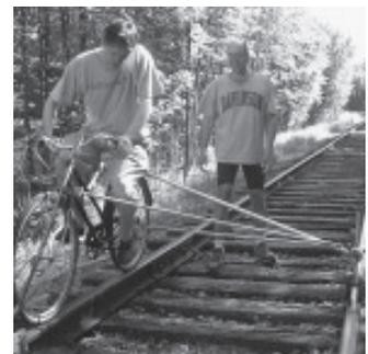
Skate wheels in a bracket attached to front wheel run against each side of rail, holding the bike in place.
