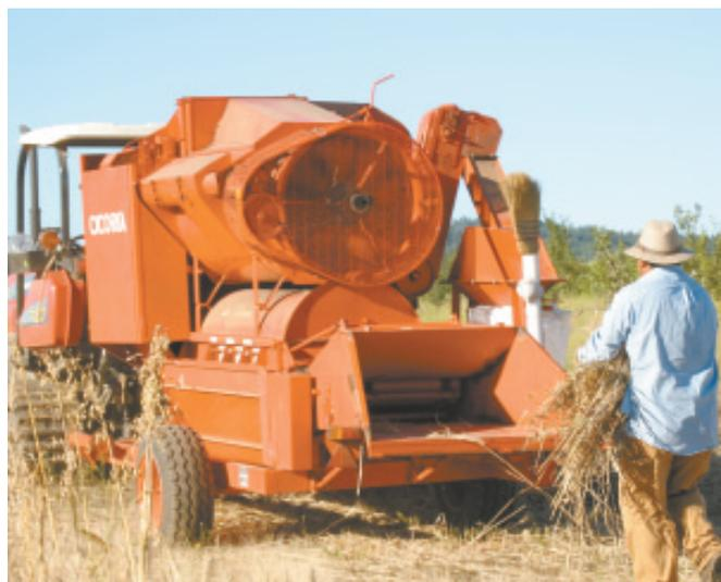
Small pto-driven thresher requires only a 45 hp tractor for power. It can be equipped with a straw cutting/crushing unit.
