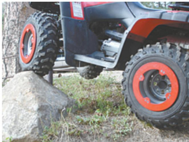
Wheel-mounted poly rings are designed to prevent damage to ATV's wheel rims. Rings extend about 1/2 in. above the rim to protect bead area of tire.
