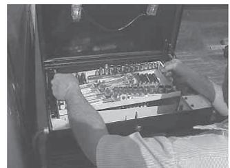
**Tool Turn toolbox is fitted with 4 by 12 by 21-in. trays. A toggle switch is used to rotate the trays.**
