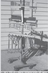
"Tool Tree" rides on four caster wheels and is made from metal pipe with wooden cross
