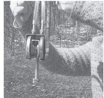
Clear hose runs from a small compressor up to the track rollers. A small shot of air is all it takes to oil the track.
