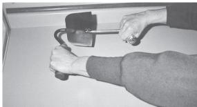
Two-handled edger uses garden hoe blade to cut.
